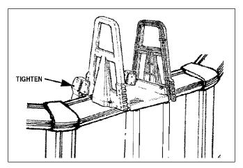
**INSTALL LADDER STEPS** (OUTSIDE POOL) Position the "outside pool" ladder steps against the handrails, aligning two ladder clevis holes with two of the holes in the handrail mounting area at each side and loosely assemble with 3/8" x 2-3/4" screws, washers and acorn nuts.
