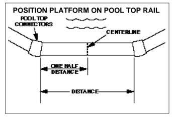
Position the platform and handrail assembly on the top rail, centered on the centerline.
