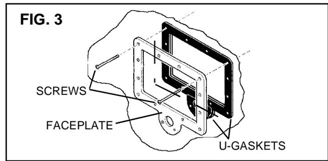
5. Position the faceplate over the gaskets and insert two large self-threading screws into the top corner holes and carefully push the screws through the holes which have been pierced in the liner. See Fig. 3.
