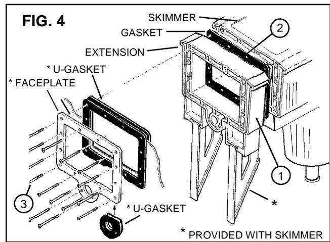
7. Insure that both inside and outside gaskets are aligned and in contact with the flanges of the faceplate, extension, and skimmer. Using the faceplate as a guide, pierce the remaining 13 screw holes in the liner. Insert the remaining screws just enough that the screw threads begin to thread into the skimmer/skim filter body. Firmly tighten all screws evenly, alternating left to right and top to bottom, until all screws are tight.
